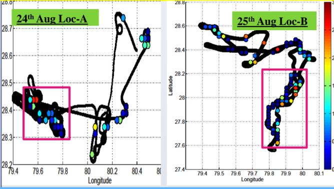
Figure 1 shows the flight path on 24<sup>th</sup> and 25<sup>th</sup> in black dots. The colored dots are total hydrometeor mass conc. (g/cubicmetre). Two regions (pink boxes) are studied where aircraft measurements are present upto 7 km altitude.
