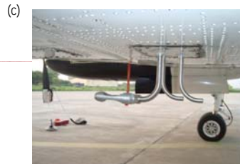
Fig 1 (a) Map of India showing the regions covered during the study, (b) aircraft with team and (c) cockpit inlet probe.
