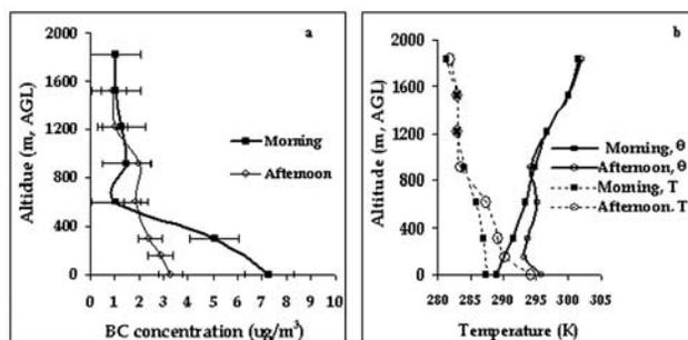
**Figure 2.** (a) Vertical profiles of BC concentration and (b) vertical profiles of temperature ( $T$ ) and potential temperature ( $\theta$ ) in experiment 1. The error bars represent  $\pm 1$  standard deviation of the corresponding measurements.
